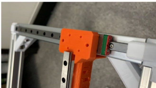
Above: the part is undersized due to plastic shrinkage, I learned to deliberately oversize the printed parts in order to compensate.
